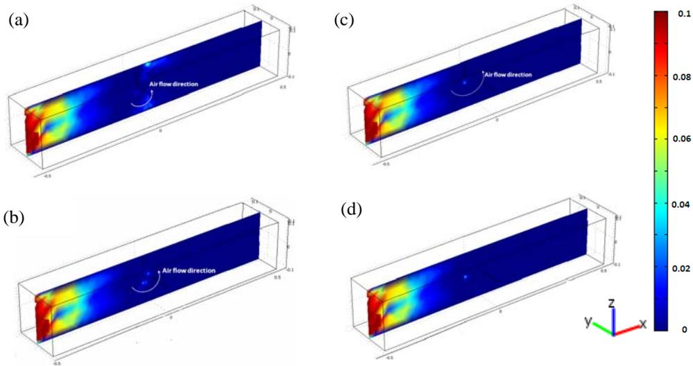
Fig.3 Swirling flow in various  $l$  when  $h = 1$  cm (a)  $l = 2$  cm; (b)  $l = 4$  cm; (c)  $l = 6$  cm; (d)  $l = 8$  cm
