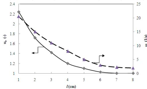
Fig.4 The maximum velocity ratio ( $u_r$ ) and vorticity ( $\omega$ ) in various  $l$
