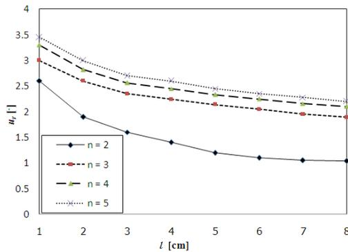
Fig.7 The maximum velocity ratio ( $u_r$ ) in various  $l$  and  $n$
