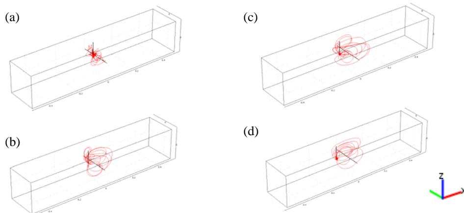
Fig.2 Electric field in various  $l$  when  $h = 1$  cm (a)  $l = 2$  cm; (b)  $l = 4$  cm; (c)  $l = 6$  cm; (d)  $l = 8$  cm
