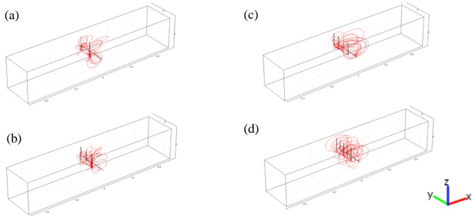
Fig.5 Electric field in various  $n$  when  $h = 1$  cm and  $l = 4$  cm (a)  $n = 2$ ; (b)  $n = 3$ ; (c)  $n = 4$ ; (d)  $n = 5$
